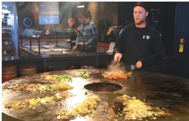
That hot grill, by the way, is a 650,000 BTU multi-burner gas griddle weighing 2,200 pounds. The Grill Warriors (cooks) carefully monitor the cooking temperatures to ensure they are maintained between 550° to 750° F.
